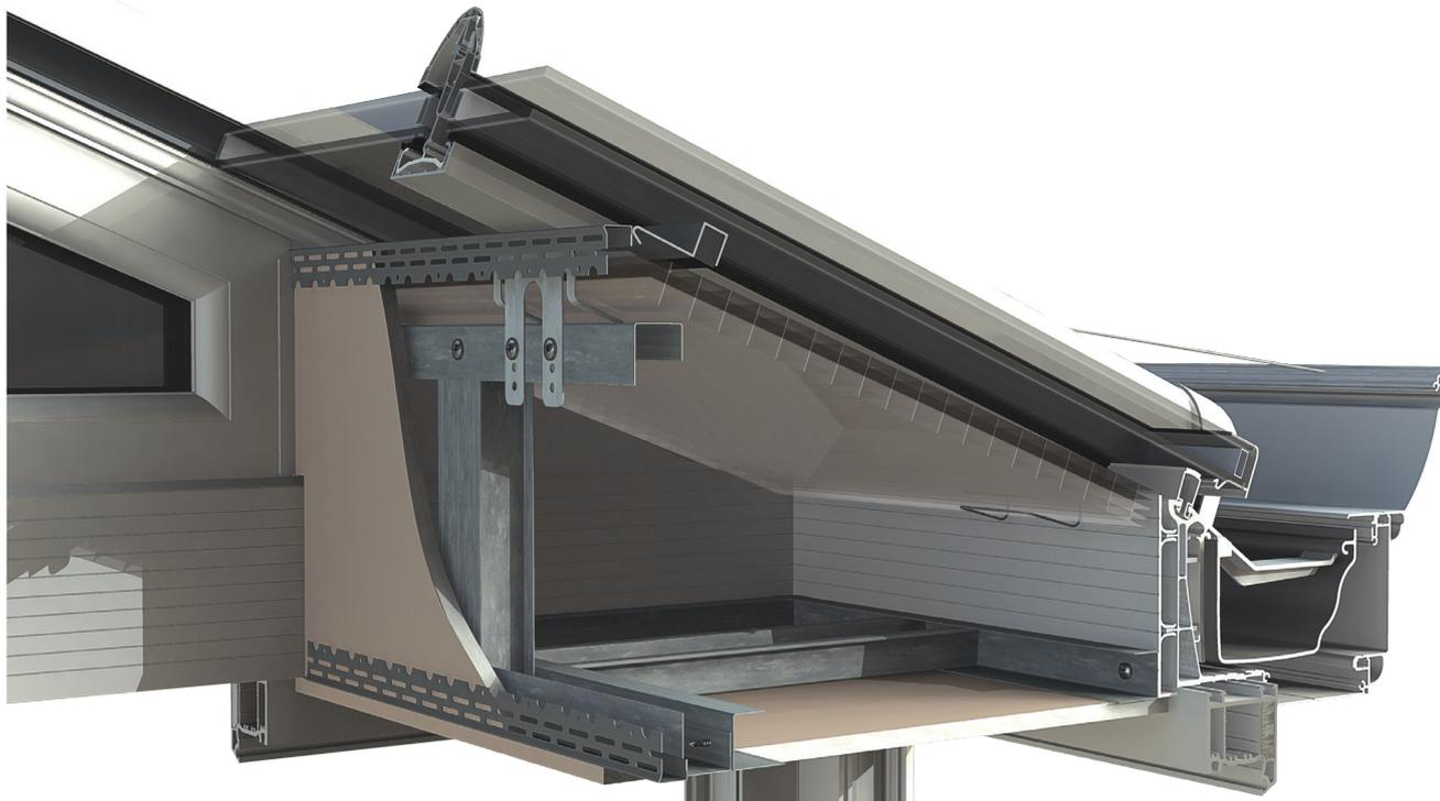
If this is a new installation of an insulated internal pelmet then the design of the gable frame should cover the 'open end' of the ladder framework. On retro fits where a redesign of the gable feature is not feasible, the application of a privacy film to the glass may suffice.
