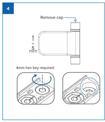
4 Height adjustment: Using a 4mm hex key turn the screw down to lift the hinge by up to 5mm.
