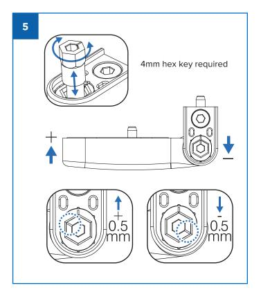
5 Compression adjustment: Push out hinge and turn to alter compression pin
