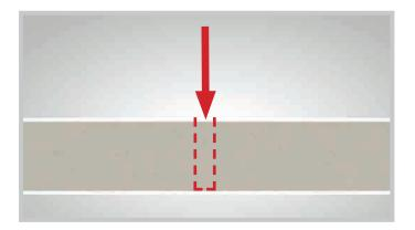
Insert your 42mm coated screw into hole and secure tightly to lower skin PVC.
