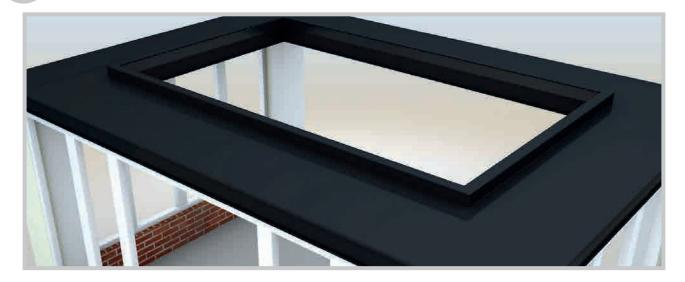
'if using epdm to cover the leka outer board you may wish to apply the following method to help a seamless finish without showing the screw dip within the roof structure when the screws are fixed in place.
