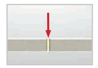
Once the EPDM finish has been applied, a trim is then fixed covering the overlap of the EPDM onto the bracket fixed in step 5a. The trim will help to further weatherproof the finish and provide extra stability to the edges of the EPDM
