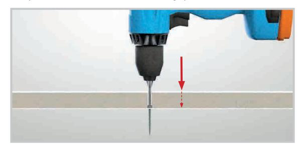
You will be provided with a foam coil which you should cut down to the appropriate length and then insert into the hole that you have drilled. Push down tightly and then your EPDM (once applied) will secure fully in place.
