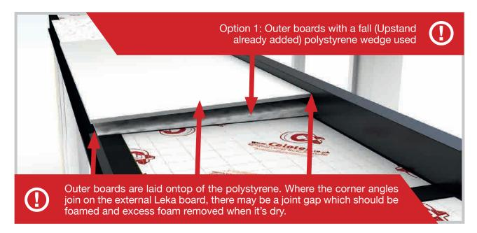
if no fall has been chosen for the Orangery roof, then the outer boards will need to be overlapped onto the inner ladder GRP. This will allow the upstand profiles to sit ontop of the outer boards sandwhiching them between the ladder GRP and the upstand profile.
