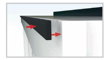
An EPDM or equivalent finish will need to be added to fully weatherproof the orangery. Please refer to you installers guide for whichever solution is being provided here.
